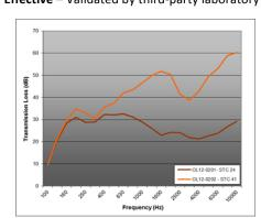
OL 12-0202 – Reference wall before application of Green Glue Noiseproofing Sealant – STC 24
